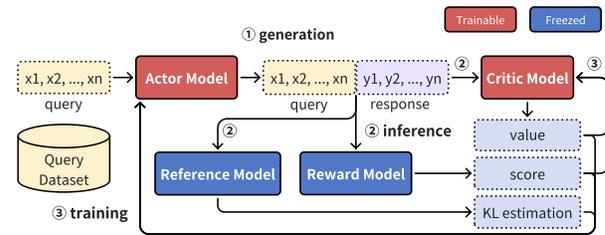
Fig. 10: An example of RLHF. **Inference process:** ① The actor model generates a response from a given query. ② The critic model, reward model, and reference model use the query and response pairs to generate the value, score, and KL divergence required for training through inference. **Training process:** ③ The actor model and critic model use the data collected in the inference process to update their weights through gradient descent.
